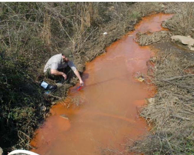
Nelson Brooke (author) tests pH & conductivity downstream of Metalplate's polluted discharge. Photo by Charles Scribner
