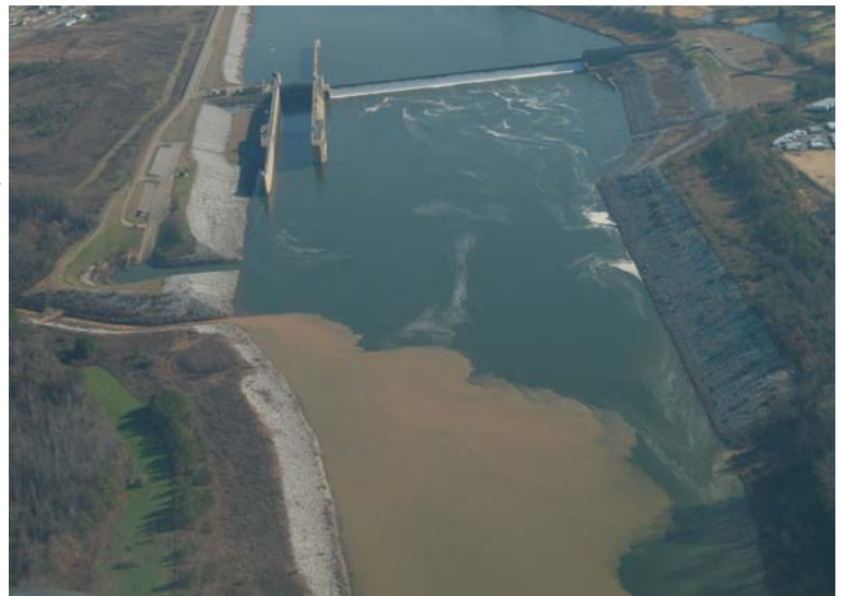
Erosion from poor development practices in the Mill Creek watershed upstream (see previous picture) cause Mill Creek to discharge incredible amounts of sediment into the Black Warrior River below Oliver Dam after rains.
